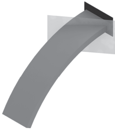
Fig. 11. Schematic representation of the specimen configuration after the bending operation, including the trimming plane.
