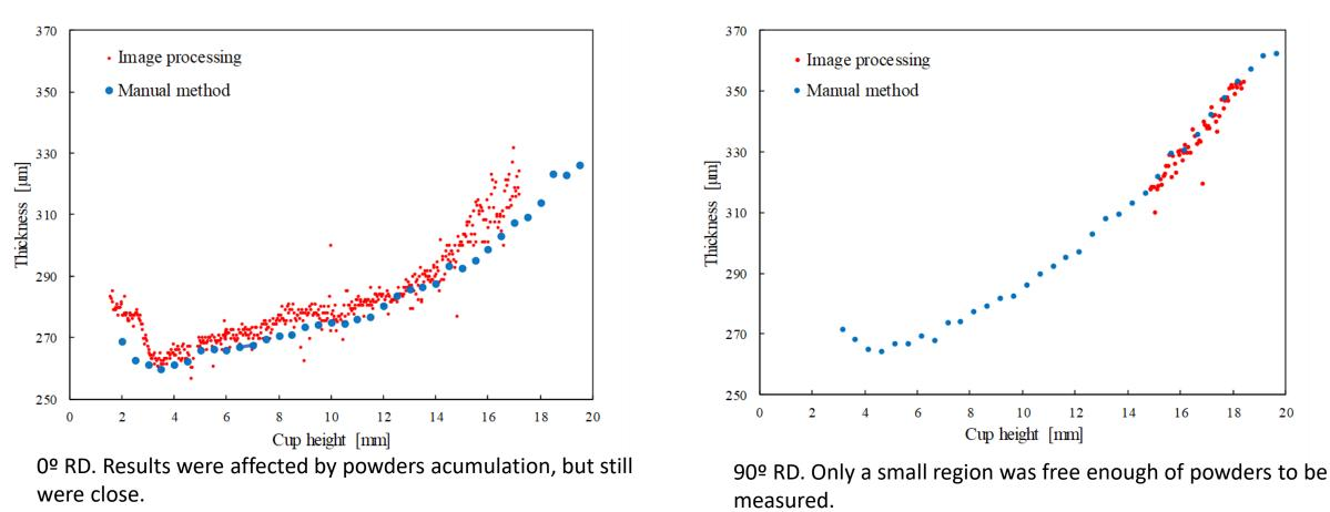
The used resin did not stick firmly, thus powders were trapped in the rift between metal and resin during polishing. This highly affected the results.
