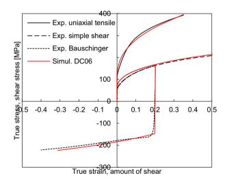
**Figure 4.** Comparison of the stress-strain curves predicted by the material model with the experimental ones for uniaxial tensile test, simple shear and Bauschinger simple shear after 20% forward shearing [26].
