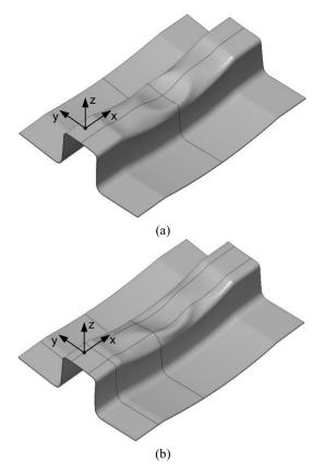
**Figure 9.** Final geometry of the rail after springback predicted by finite element simulation: (a) 1/4 of blank; (b) full blank including the four cross-sections used to evaluate the geometrical defects.
