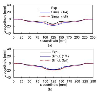
**Figure 11.** Comparison between experimental and numerical profile of the cross-section: (a) L1 (y=0 mm); (b) L2 (y=-30 mm).
