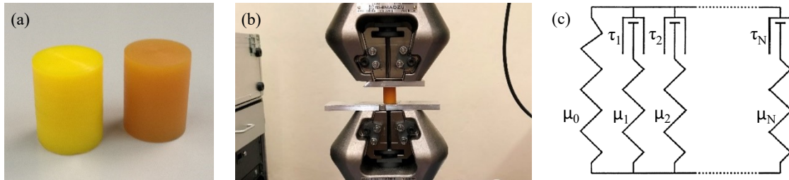
FIGURE 1. Experimental apparatus and constitutive model: (a) rubber specimens; (b) grips of the universal tensile testing machine; (c) generalized Maxwell model.
