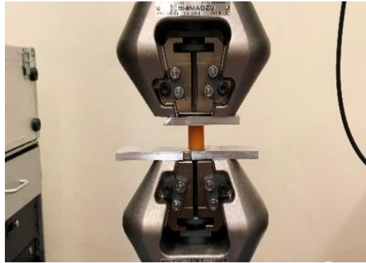
Figure 3. Experimental apparatus used for the uniaxial compression test under quasi-static loading.
